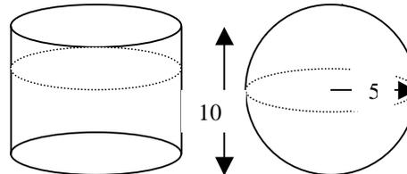
The cylinder is drawn for comparison. We know the volume of the cylinder = area of base x height =  $(\pi r^2)(h) = 3.14(25)(10) = 785$  cubic units (approx). Therefore, the volume of the sphere =  $(\frac{2}{3})(785) = 523.3$  cubic units.
