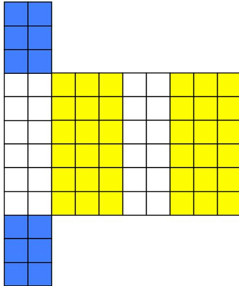
This **pattern** would fold up to make the prism pictured above. The white 2 by 6 rectangles would cover the front and back. The yellow 3 by 6 rectangles cover the right and left faces. The blue 2 by 3 rectangles cover the top and bottom. Total surface area =  $2(2 \times 6) + 2(3 \times 6) + 2(2 \times 3) = 72$  square units.
