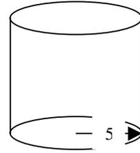
The cylinder is drawn for comparison. We know the volume of the cylinder =  $\pi r^2(h) = 3.14(25)(8) = 628$  cubic units (approx).
