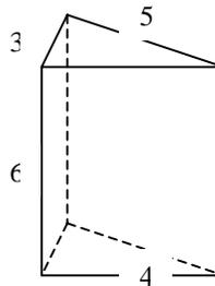
Since the triangle is a right triangle we know its base and height, 4 units and 3 units. Thus, the base area =  $0.5(4 \times 3) = 6$  square units. The height of the prism is 6 units. Therefore, the volume of the prism = base area x height =  $6 \times 6 = 36$  cubic units.
